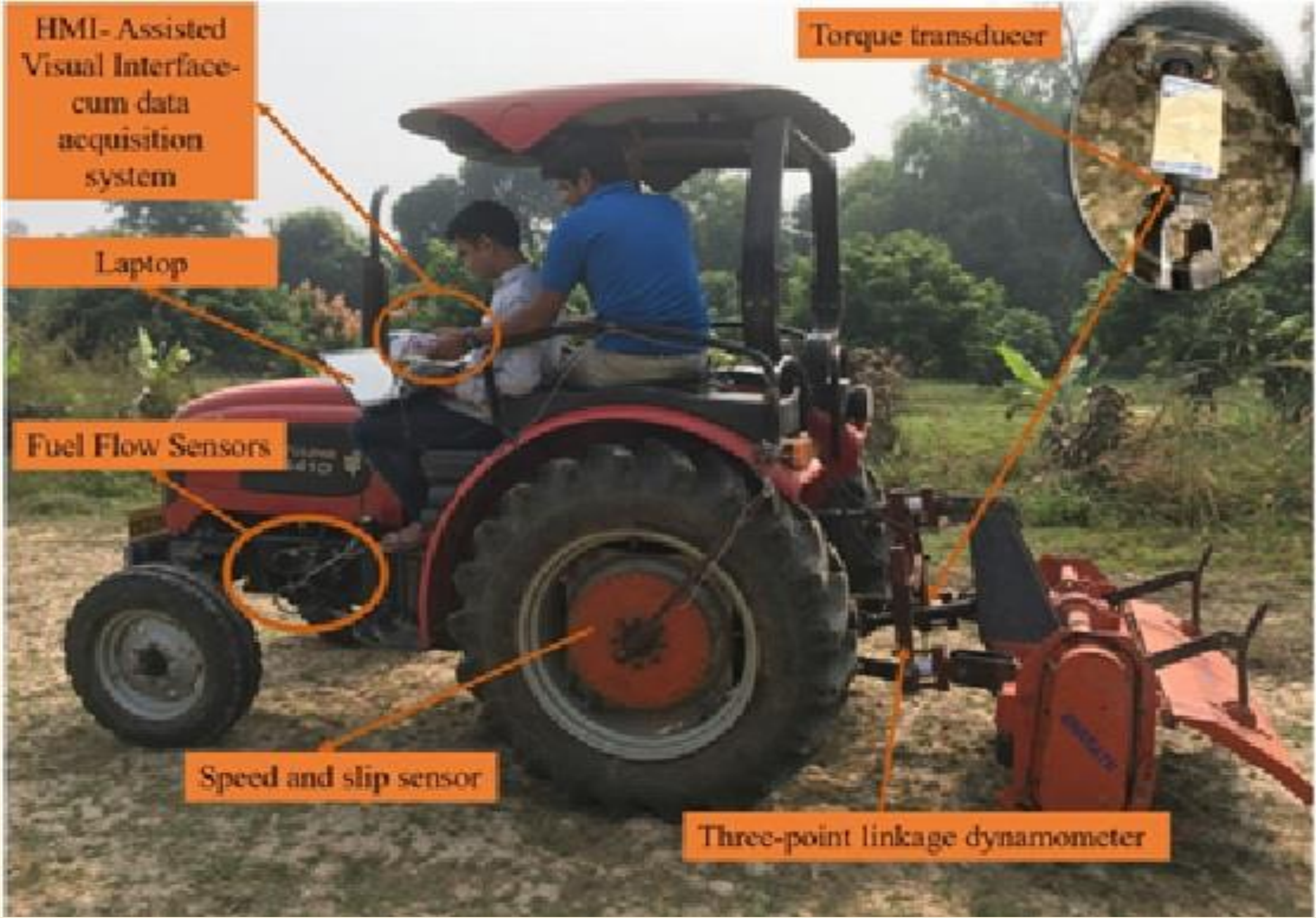
Testing the system developed with rotavator. HMI, human-machine interface. Source: wileyonlinelibrary.com
